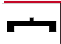
Part. 263 - Page 6 Chain guide profile. Multiple strands K82,5 / pitch 88
