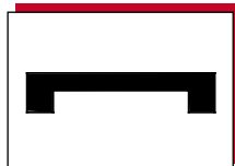
Part. 387 - Page 7 Chain guide profile. Multiple strands K87 / pitch 88
